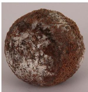
When sponges are removed from the cage after use, clean out feed residues and grease immediately. If the sponges are left moist and dirty over time, fungus and mould will grow in them. If they are sent through the feeding pipes without being perfectly cleaned or containing residues from fungus or mould, this may infect the feed, risking contamination of the fish.
