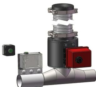
The green buttons are placed next to the Motorized Feed Pipe Cleaner and in the control room, and are marked with what they do, and of which feed line they control the cleaning.
